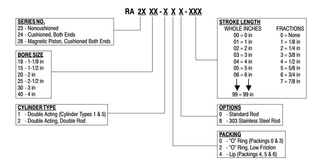
NOTE: Reciprocating assembly is furnished assembled with all required components, less seals. It is recommended that new seal kits be used when replacing reciprocating assemblies. See below for Seal Kit requirements.
